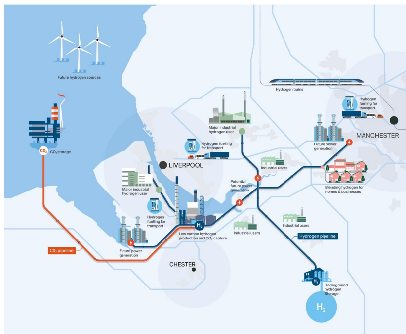
Figure 2: Hynet will produce, store and distribute hydrogen as well as capture and store carbon dioxide from industry in the Northwest of England and North Wales
